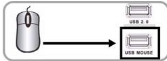
Figure 1.0 Connect a USB mouse to the bottom USB port on the rear panel
